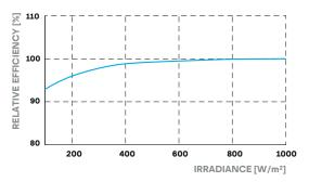
Typical panel performance under low irradiance conditions in comparison to STC conditions (  $25^{\circ}$ C, 1000 W/m<sup>2</sup>).
